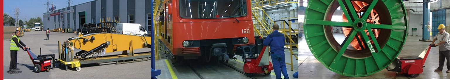
The Original **Power Pusher**<sup>®</sup> is a pedestrian operated electric tug. It's capable of pushing and pulling loads up to 40,000kg, subject to the rolling resistance of the load. The Power Pusher<sup>®</sup> has been in continuous production for more than 50 years, during this time over 100 application-specific attachments have been developed.
